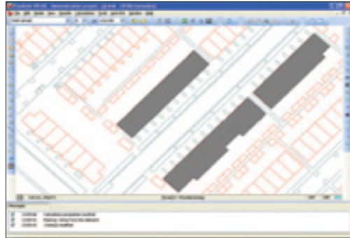
Fig. 4 (Left) Model view with multi-layer DXF background as snap option for items (buildings, roads etc.), enabling faster modelling Fig. 5 (Right) Model view of Arnhem, Holland, with 70,000 buildings and 2500 roads on a satellite image as background
